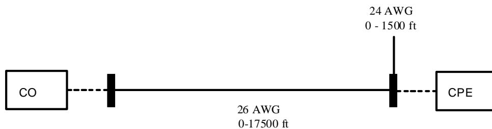
Figure 12: Bridged Tap Loop Configuration
