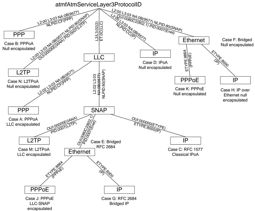
**Figure 1: Tree representation of access protocols and encapsulations**
